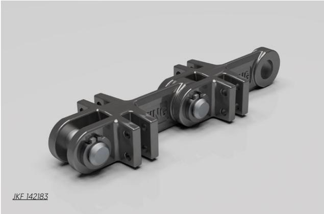
Where extra wide flights are required the John King triple link is available allowing, in conjunction with the double on perimeters, three chain strands up to 3100 mm overall. In addition the "Double slot" allows for a versatile means of flight retention for both steel & plastic options. Retention can be either U clips or standard fasteners.
