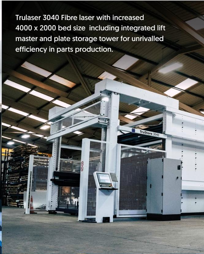
Trulaser 3040 Fibre laser with increased 4000 x 2000 bed size including integrated lift master and plate storage tower for unrivalled efficiency in parts production.
