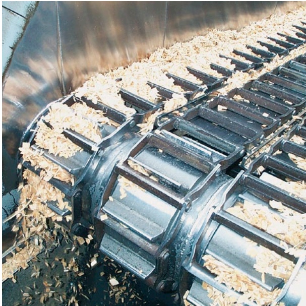
Articulation is Between Chain Barrel and Sprocket Tooth
